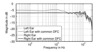
**Figure 3:** Averaged and weighted magnitude responses over the full sphere for the left and the right ear with and without the common diffuse field compensation filter (common DFC).
