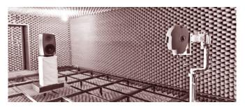
Figure 1: Genelec 8260A speaker and Neumann KU100 dummy head mounted on the VariSphear motion system [5] in the anechoic chamber. [Photo: P. Stade]
