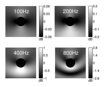
Figure 4: Analytic simulation of the pressure magnitude at different frequencies for a plane wave impact with unit gain from south to a rigid sphere with a typical diameter of 17.5 cm serving as a simplified model of the dummy head. Below the LFE crossover frequency of 200 Hz, the magnitude deviations on the sphere surface are already less than  $\pm 0.2$  dB.
